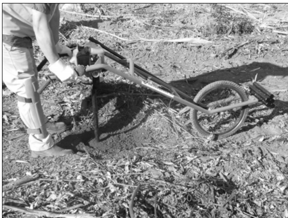
Figure 3. Hand held motorised auger with improved ergonomic design.
