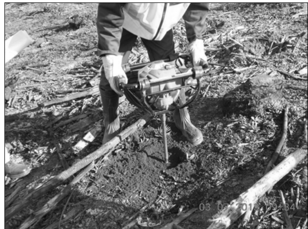
Figure 2. Hand held motorised auger.
