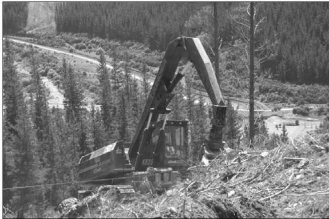
Figure 1. ClimbiMAX felling machine with winch integrated into chassis.
